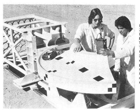
DEAN JACOBY (MAN-ZANO LABS) AND LEROY PEREA (9335, right) CHECK ELECTRICAL CONNEC-TIONS BEFORE FIRST TEST. The 120° segment of a turbine hub weighed about 3400 pounds. Mounted on a lightweight sled, it was propelled by rockets to a speed of 320 mph. Before impact, explosive bolts decoupled the turbine segment.
